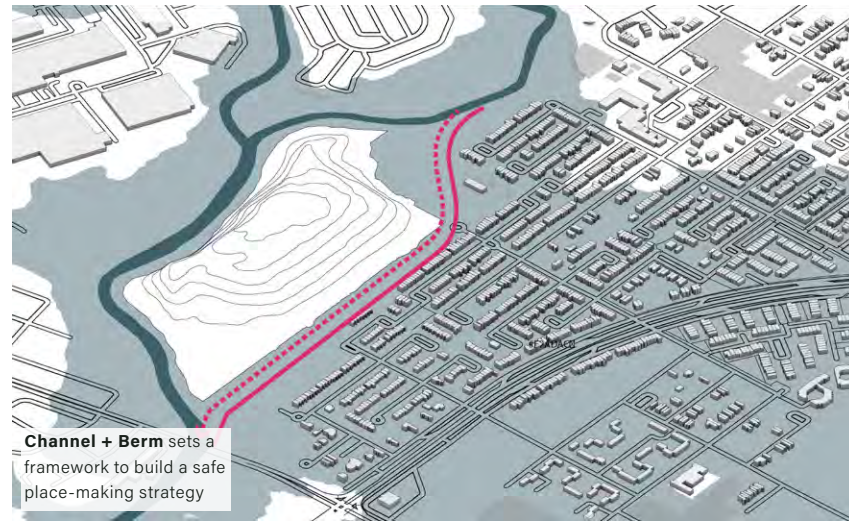
Pinch Point causes back flow of creek into Eastwick neighborhood during major storms
